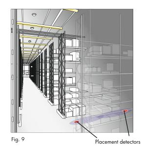
So that movement in the main aisles is not detected, half the lens (the side towards the main aisle) should be covered with blinds. There are frequently several parallel side aisles, divided from each other by open racking. Since the detector may also pick up movement from neighbouring aisles through the open racking, it is also recommended that blinds are used to filter out this area. (Fig. 9).
