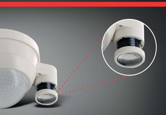
The telescopic part of the light sensor is pulled out according to the mounting height. This enables a daylight-dependant regulation to a mounting height of up to 16 m.
