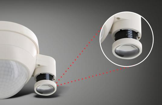
The telescopic part of the light sensor is pulled out according to the mounting height. This enables a daylight-dependant regulation to a mounting height of up to 16 m.
